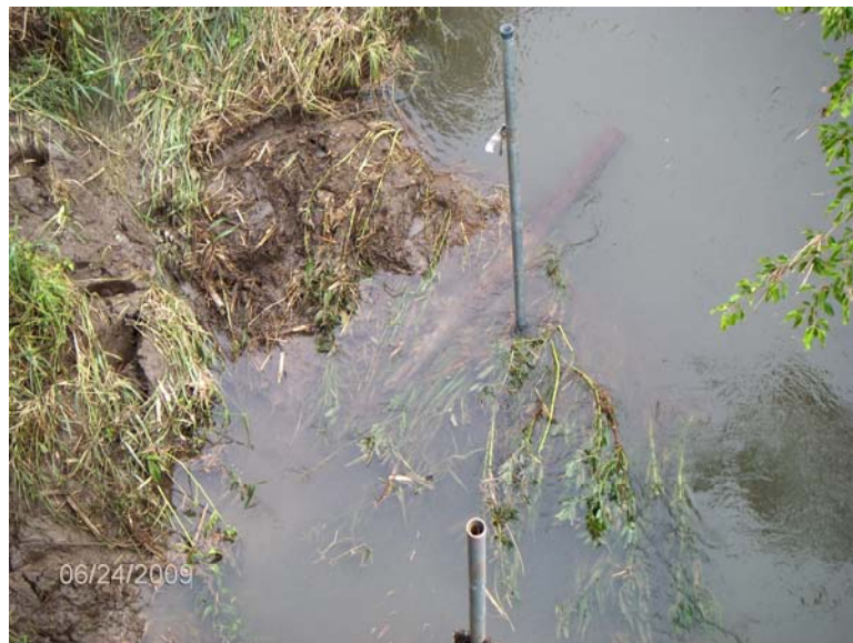
Figure 2.2: Orientation of the two pipes at the SAC site. This picture was taken looking up stream, the closest pipe has the sensors attached and the one farthest away was added as a barricade to protect the sensors. Note the sunken large wooded pole that was stopped by the first pipe.
